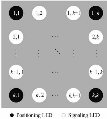
**Fig.6 Schematic diagram of  $k$ -stage LED array**
