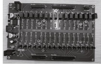
**Fig.4 Physical picture of LED array drive circuit**
