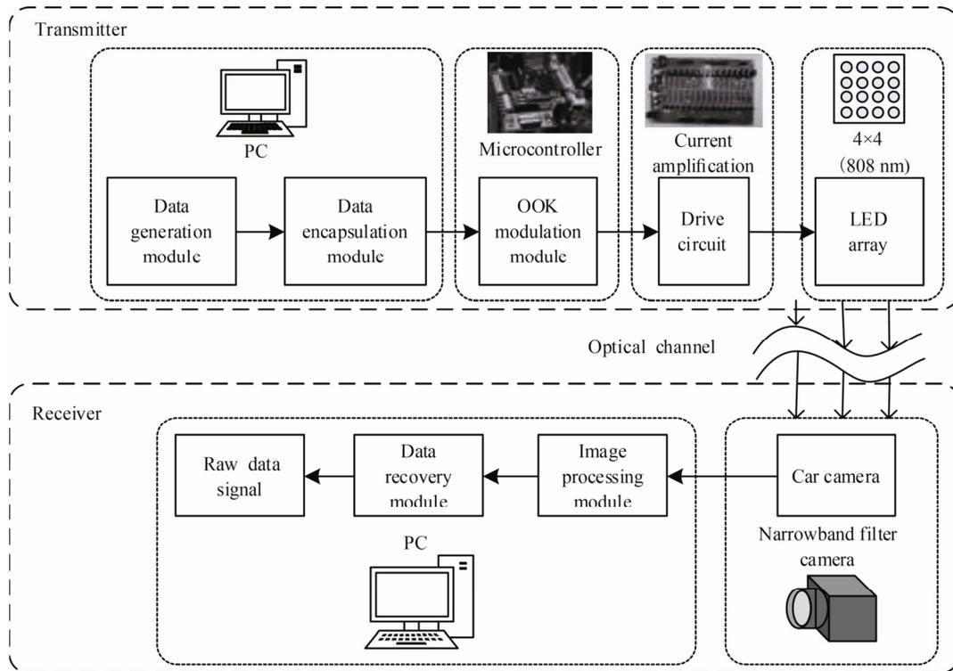
**Fig.1 The structure of MIMO-based OCC system**
