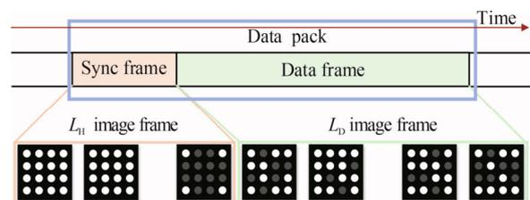
**Fig.2 Data package structure diagram**
