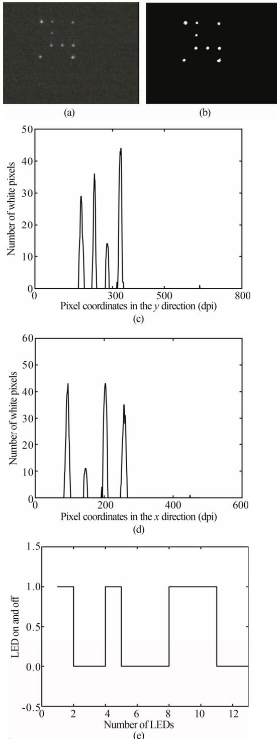
**Fig.7 Decoding process: (a) The original image; (b) Binary image; (c) Vertical projection; (d) Horizontal projection; (e) Decoding result**
