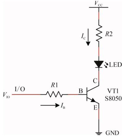
Fig.3 Schematic diagram of LED drive circuit
