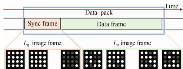
**Fig.2 Data package structure diagram**
