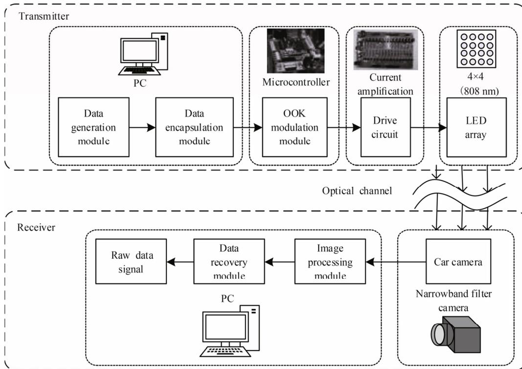
**Fig.1 The structure of MIMO-based OCC system**
