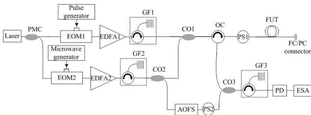
**Fig.2 Experimental setup for single-ended BOTDA system with pulse coding based on Fresnel reflection**
