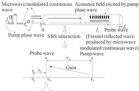
**Fig.1 Principle diagram of the heterodyne detection single-ended BOTDA system based on Fresnel reflection**
