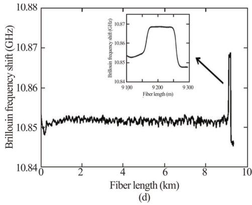
**Fig.4 Brillouin frequency shift distributions under different coding bits: (a) Single pulse; (b) 8 bit coding; (c) 16 bit coding; (d) 32 bit coding**
