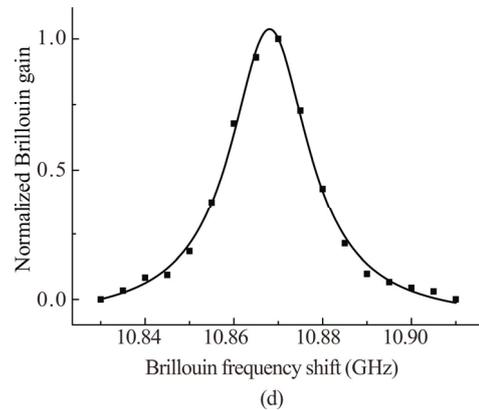
**Fig.5 Brillouin gain spectra with Lorentz fitting under different coding bits: (a) Single pulse; (b) 8 bit coding; (c) 16 bit coding; (d) 32 bit coding**
