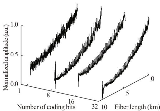
**Fig.3 Brillouin power distributions under different coding bits**
