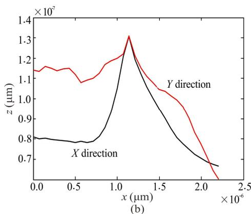
**Fig.4 Effect diagrams of AFM tip reconstruction: (a) Three-dimensional effect; (b) Two-dimensional effect**
