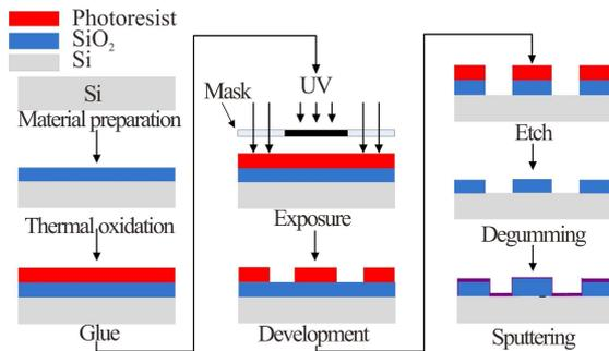
Fig.1 Preparation process of the lattice sample
