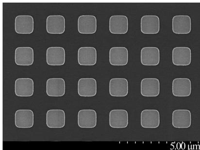
Fig.2 The 2 μm lattice sample under SEM
