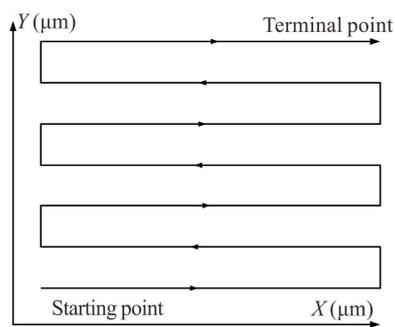
**Fig.3 AFM probe scanning route**
