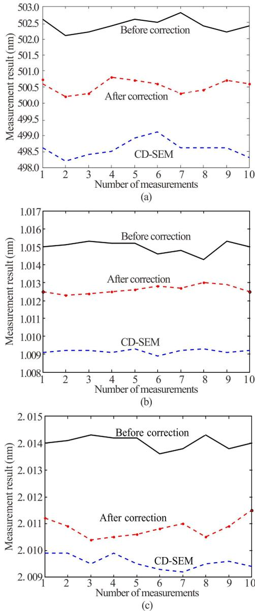
**Fig.6 Measurement results before and after correction with different nominal values: (a) 500 nm; (b) 1  $\mu\text{m}$ ; (c) 2  $\mu\text{m}$**
