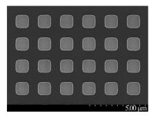
Fig.2 The 2 µm lattice sample under SEM
