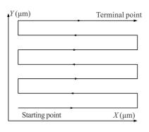
Fig.3 AFM probe scanning route
