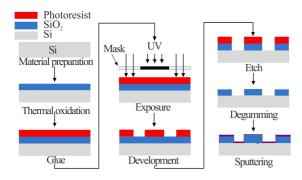
Fig.1 Preparation process of the lattice sample
