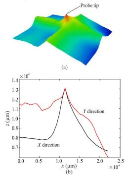
Fig.4 Effect diagrams of AFM tip reconstruction: (a) Three-dimensional effect; (b) Two-dimensional effect
