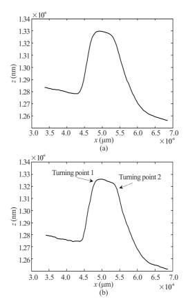
Fig.5 Measurement curves of AFM: (a) Before probe correction; (b) After probe correction
