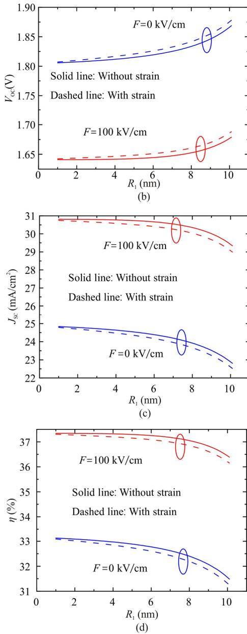
**Fig.2** The QD (a) band gap, (b)  $V_{oc}$ , (c)  $J_{sc}$ , and (d)  $\eta$  as a function of QD core size  $R_1$  with and without strain for In content  $x=0.3$ , QD shell size  $R_2=15$  nm, and external electric field  $F=0, 100$  kV/cm
