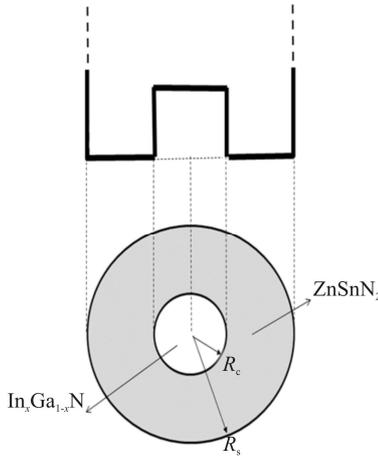
**Fig.1 Schematic diagram of In<sub>x</sub>Ga<sub>1-x</sub>N/ZnSnN<sub>2</sub> core/shell spherical QD**
