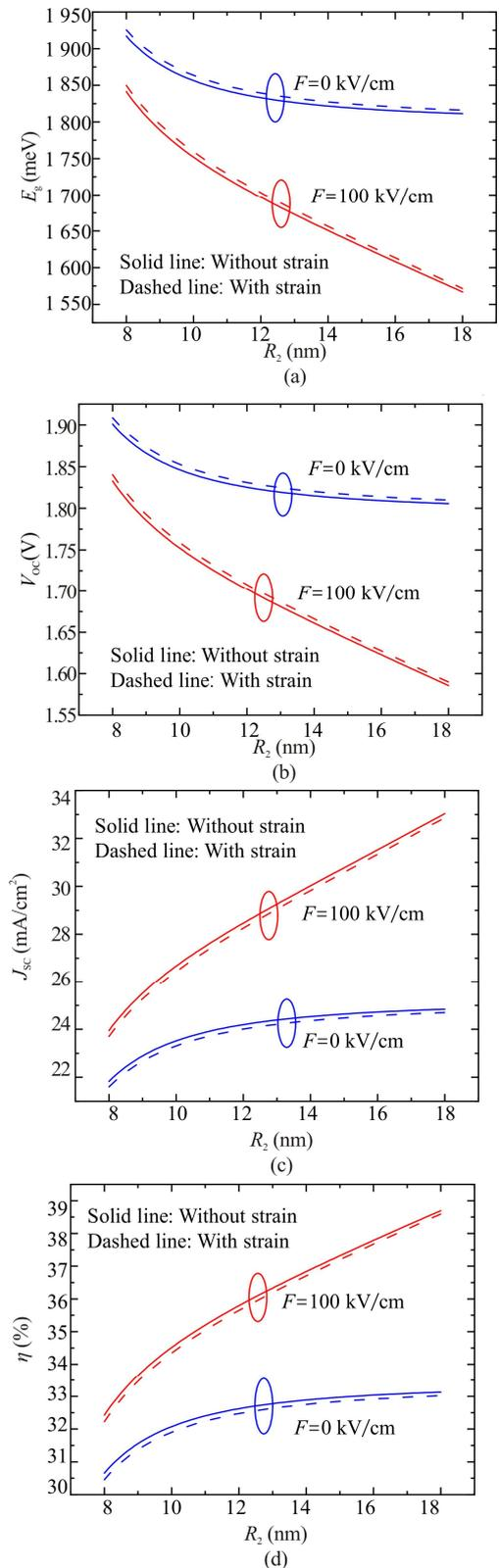
**Fig.3** The QD (a) band gap, (b)  $V_{oc}$ , (c)  $J_{sc}$ , and (d)  $\eta$  as a function of QD shell size  $R_2$  with and without strain for In content  $x=0.3$ , QD core size  $R_1=4$  nm, and external electric field  $F=0, 100$  kV/cm
