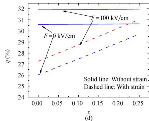
**Fig.4** The QD (a) band gap, (b)  $V_{OC}$ , (c)  $J_{SC}$ , and (d)  $\eta$  as a function of In content  $x$  with and without strain for QD core size  $R_1=4$  nm, shell size  $R_2=7$  nm, and external electric field  $F=0,100$  kV/cm
