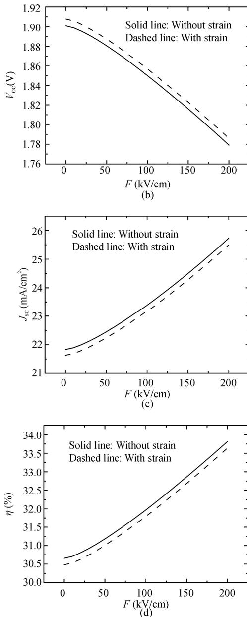
**Fig.5** The QD (a) band gap, (b)  $V_{oc}$ , (c)  $J_{sc}$ , and (d)  $\eta$  as a function of external electric field with and without strain for In content  $x=0.3$ , core size  $R_1=3$  nm, and shell size  $R_2=7$  nm
