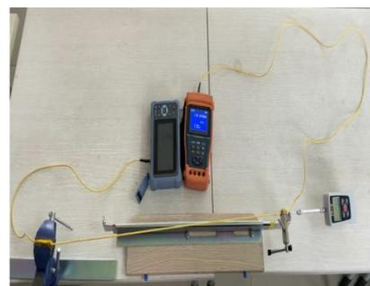
**Fig.3 Layout of straight-pull fiber tensile test**
