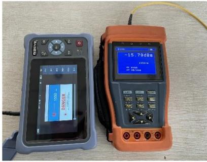
**Fig.4 Optical power meter**
