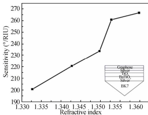
**Fig.2 Variation of sensitivity with respect to analyte refractive index**
