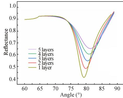
**Fig.3 Reflectance versus angle of incidence with different graphene layers at wavelength of 633 nm**
