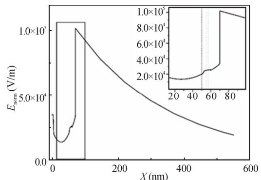
**Fig.4 Electric field distribution at resonance angle of SP wave in the proposed sensor at wavelength of 633 nm (Inset: zoomed section of the electric field)**
