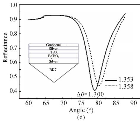
**Fig.1 Reflectance versus angle of incidence with different layer configurations for (a) Ag/Ag, (b) Ag/BaTiO<sub>3</sub>/Ag, (c) Ag/BaTiO<sub>3</sub>/Ag/graphene, and (d) Ag/BaTiO<sub>3</sub>/TiO<sub>2</sub>/Ag/graphene**
