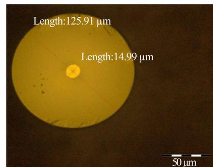
**Fig.1 Microscopic cross-sectional view of the fiber (BDF-SA)**
