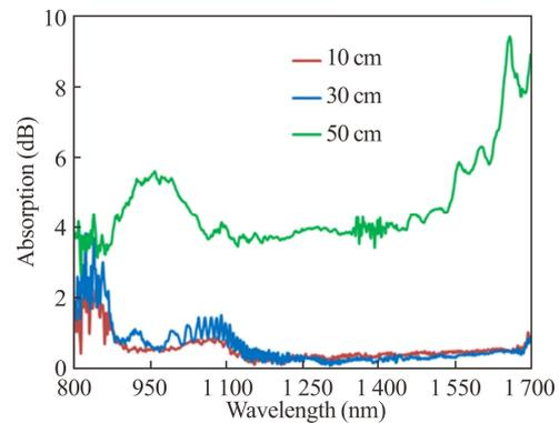
**Fig.3** Linear absorption spectra of BDF with different lengths
