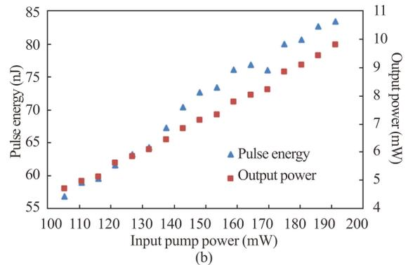
**Fig.6 Q-switched laser performance at various launched pump power: (a) Measured pulse width and repetition rate; (b) Pulse energy and average output power**
