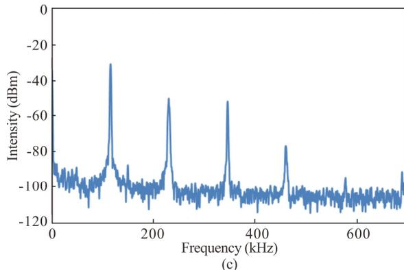
**Fig.5 Q-switched laser characteristics: (a) Output spectra; (b) Typical oscilloscope trace; (c) RF spectrum**
