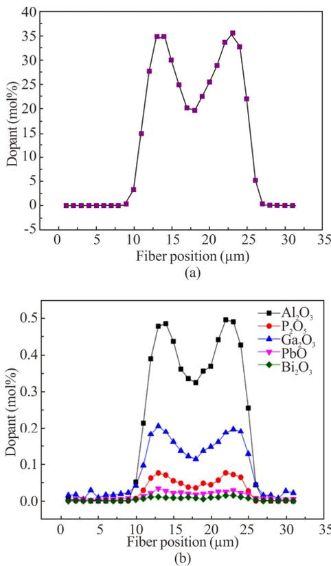
**Fig.2** Distribution curves of (a)  $\text{GeO}_2$  and (b) other oxide elements, such as  $\text{Al}_2\text{O}_3$ ,  $\text{P}_2\text{O}_5$ ,  $\text{Ga}_2\text{O}_3$ ,  $\text{PbO}$ , and  $\text{Bi}_2\text{O}_3$  along the diameter of BDF-SA determined from EPMA
