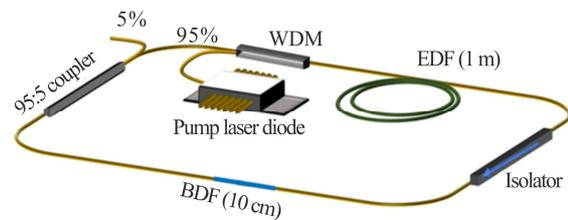
**Fig.4** Schematic arrangement of the Q-switched EDFL with BDF SA
