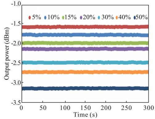
**Fig.5 Stability of the proposed sensor**
