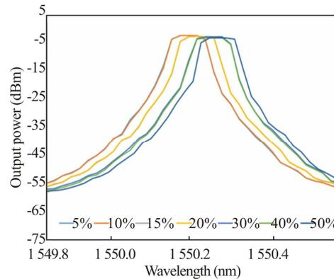
**Fig.6 Transmission spectra of the proposed sensor**
