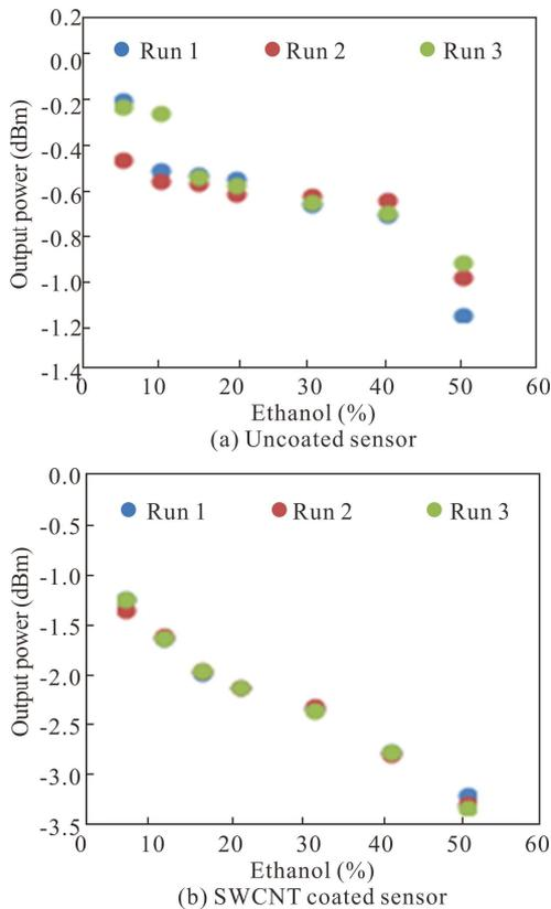
**Fig.4 Outputs of (a) uncoated and (b) SWCNT coated sensors in three different runs, respectively**
