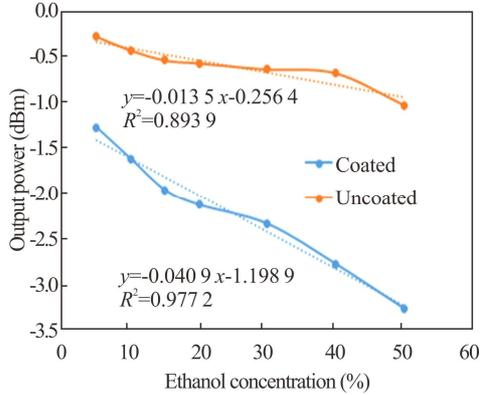
**Fig.3 Transmitted power of the sensor as a function of ethanol solution concentration**
