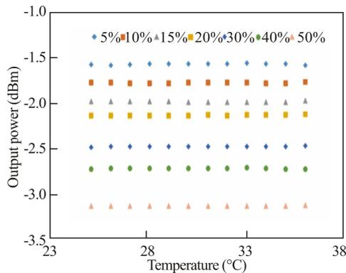
**Fig.7 Output power at various temperatures**
