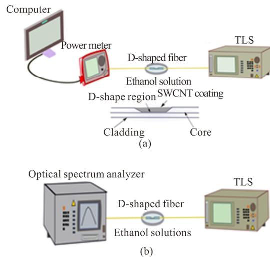
**Fig.2 Experimental setup for the ethanol sensor based on (a) power variation and (b) wavelength shift measurement**
