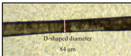
**Fig.1 D-shaped silica fiber sample coated with SWCNTs**
