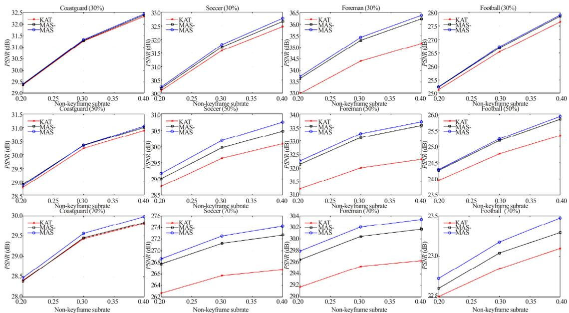
**Fig.6 Average PSNR results for different algorithms under different non-keyframe substrates and skipping ratios**
