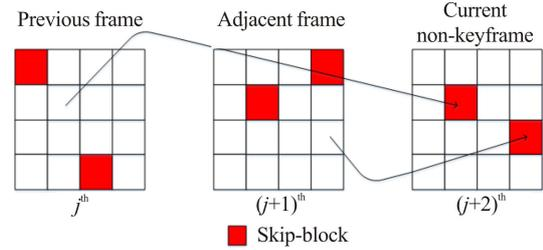
Fig.4 Skip-block measurements compensation of adjacent-reference-frame analyzing
