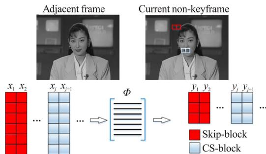
Fig.3 Diagram of adjacent-reference-frame analyzing
