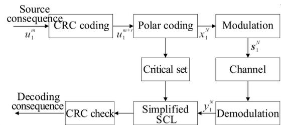
**Fig.6 Flow chart of CA-SCL coding and decoding**
