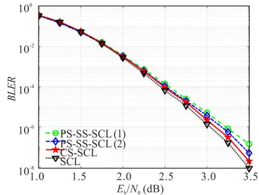
**Fig.7 BLER under different decoding schemes at  $N=1\ 024$  and  $a=20$**
