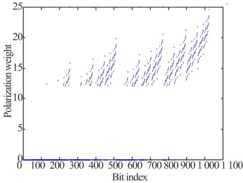
**Fig.4 Reliability of polarized channels evaluated by polarization weights**
