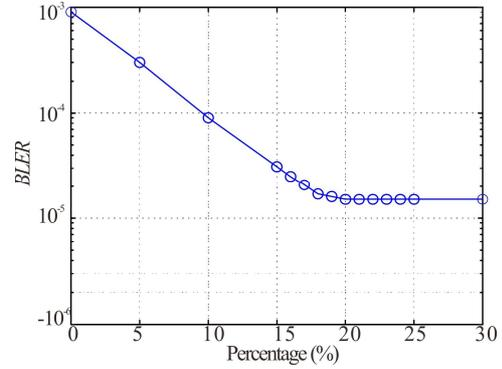
**Fig.5 BLER performance after adding low-reliability bits index to the critical set**
