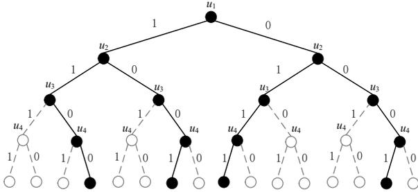
**Fig.1 Decoding tree of SCL decoding for paths reduction**
