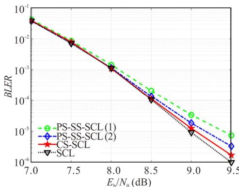
**Fig.9** *BLER* under different decoding schemes at  $N=512$  over Rayleigh fading channel
