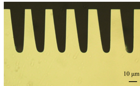
Fig.2 Partial view of the waveguide end face under a microscope
